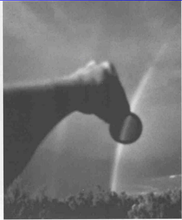
Fig. 4.8B Rotate the polaroid 90°, and the light of the rainbow is passed by the polaroid.
